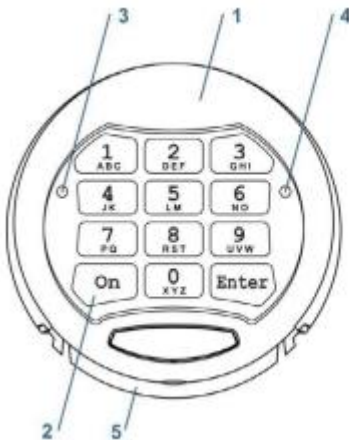
Fig. 1.1 1. Case 2. Keypad 3. Green LED [G] 4. Red LED [R] 5. Battery Box
